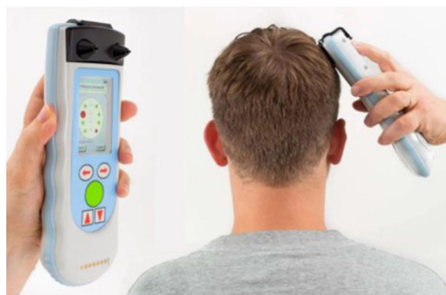
Figure 2. The Infrascanner Model 1000 is a handheld device that uses near infra-red light to detect intracranial hemorrhage
